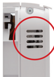
Sensor for indoor temperature and humidity
